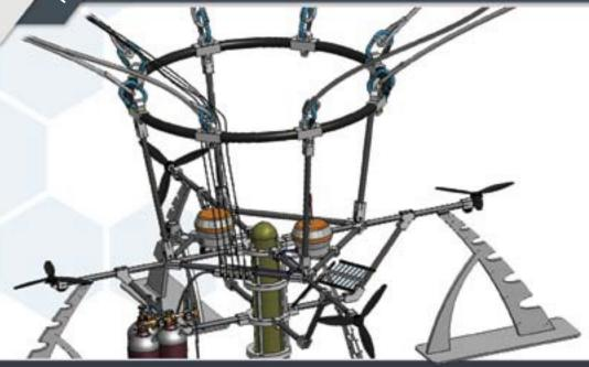
Start of a micro-rocket with a satellite from a platform floating in the stratosphere
