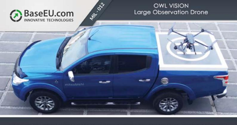
A large base observation drone measuring 220 cm x 220 cm carried on a launcher platform, built-in on a UT Mitsubishi L 200 vehicle
