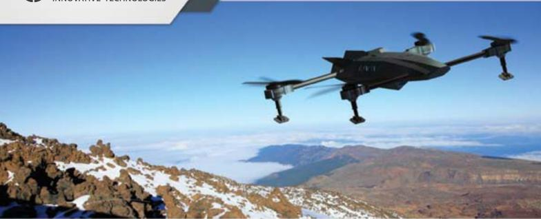
An innovative, large, multitask drone with a hybrid combustion-electric engine, based on multirotor technology
