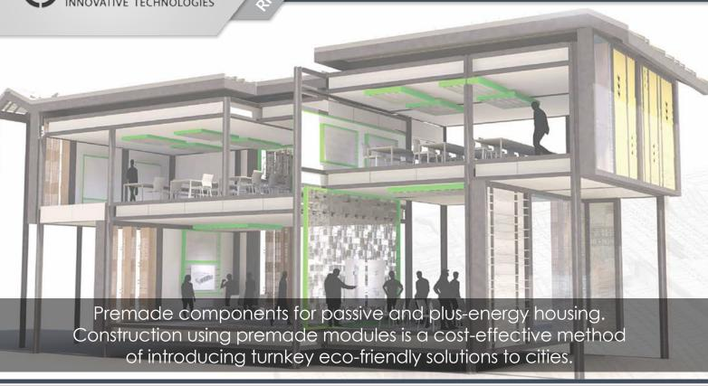
Passive housing solutions may be applied in free-standing houses as well as in large multi-family complexes and office buildings. In both cases, there is a possibility of segmental technology application. It uses closed-end, complete modules. New objects are constructed from high-quality prefabricates required in energy-saving constructions.
