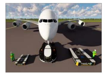
Rail technology allows almost entire coverage of transportation trolleys. They are made of high quality materials resistant to unfavourable weather conditions. Their installation is very fast – during an 8-hour pause in an airport's functioning, 250 metres of rails may be built.
